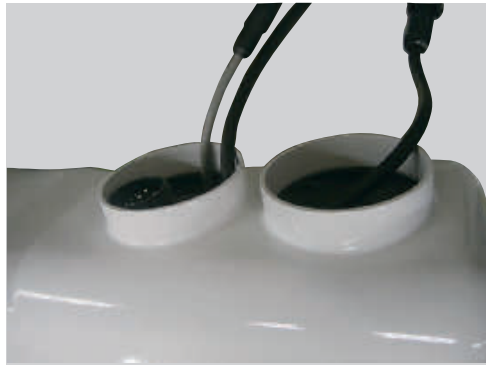
Cables removed when temporarily inserting cover
