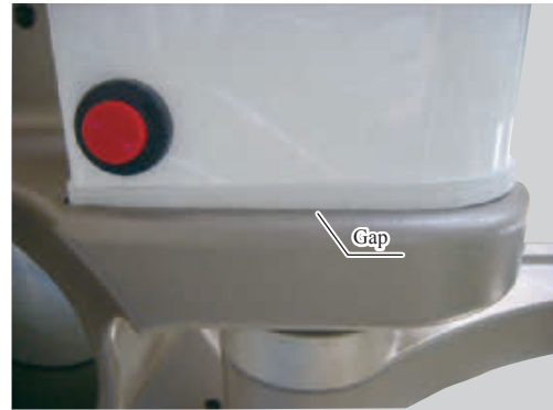
Gap at bottom of cover
